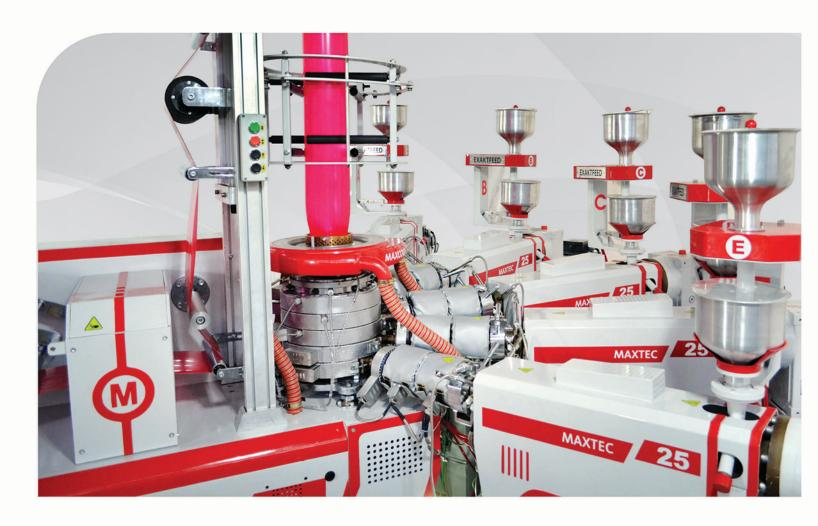
The MX-B520 belongs to the new generation of smart pilot extrusion lines. This equipment is basically dedicated for product testing and development.
