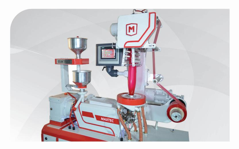
The compact and versatile blown film machine MX-B120 is a very useful tool for continuous quality check of different production batches at resin suppliers and masterbatch producers. It is also widely used for testing material properties and performance. The simple and intuitive operator interface makes the machine very user friendly and practical for every day operation.
